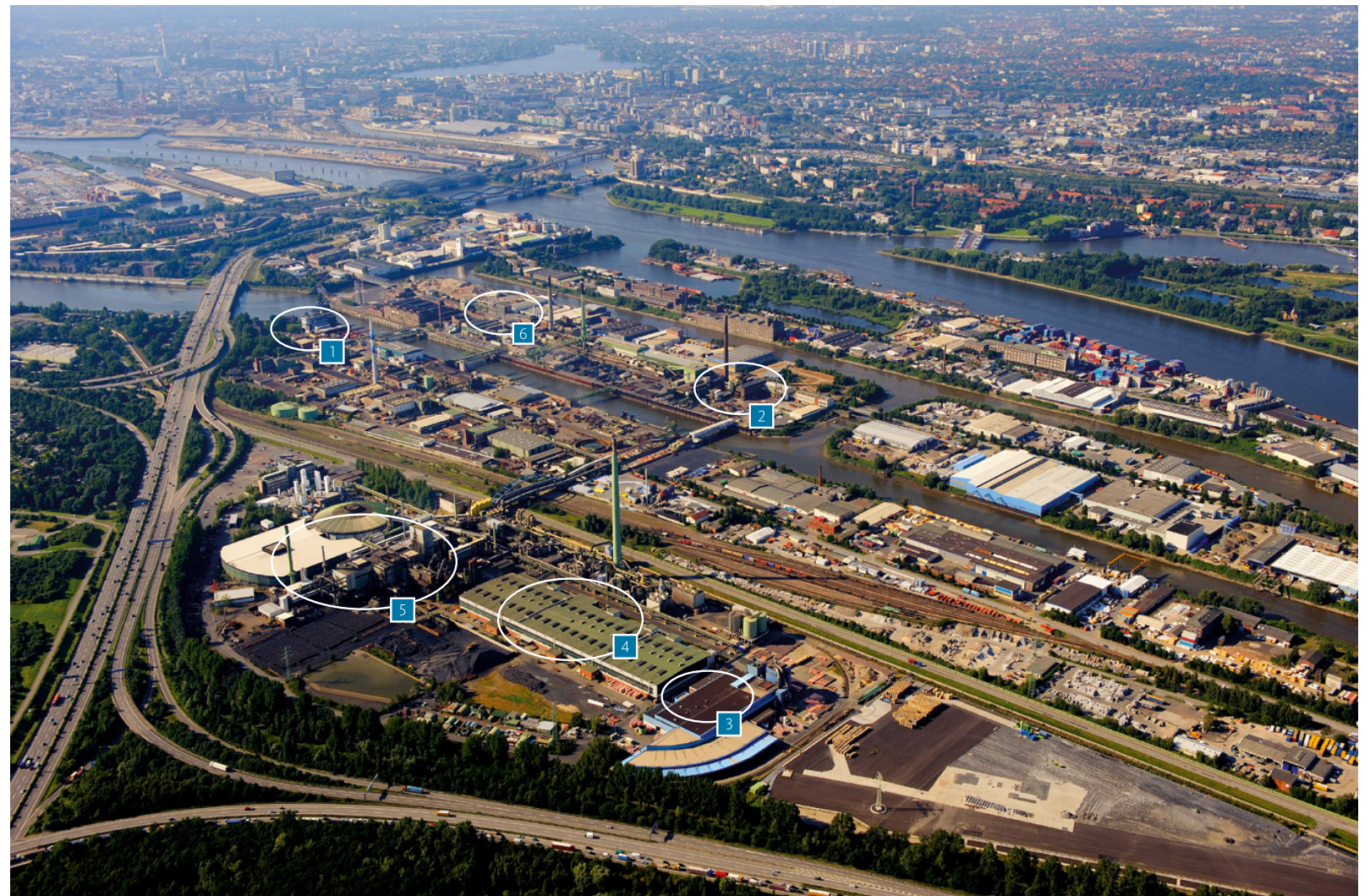
1 Continuous casting plant 2 Secondary copper smelter/precious metals 3 Rod plant 4 Tankhouse 5 Primary smelter (RWO) 6 Administrative buildings
