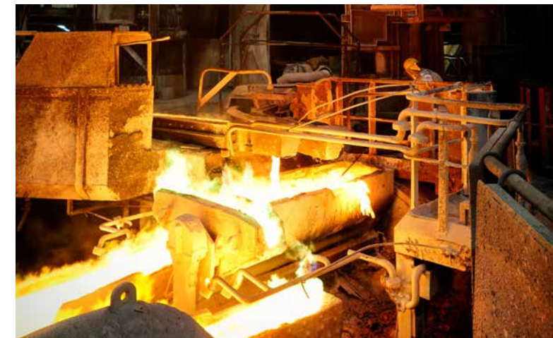
Anode casting wheel at the Hamburg plant
