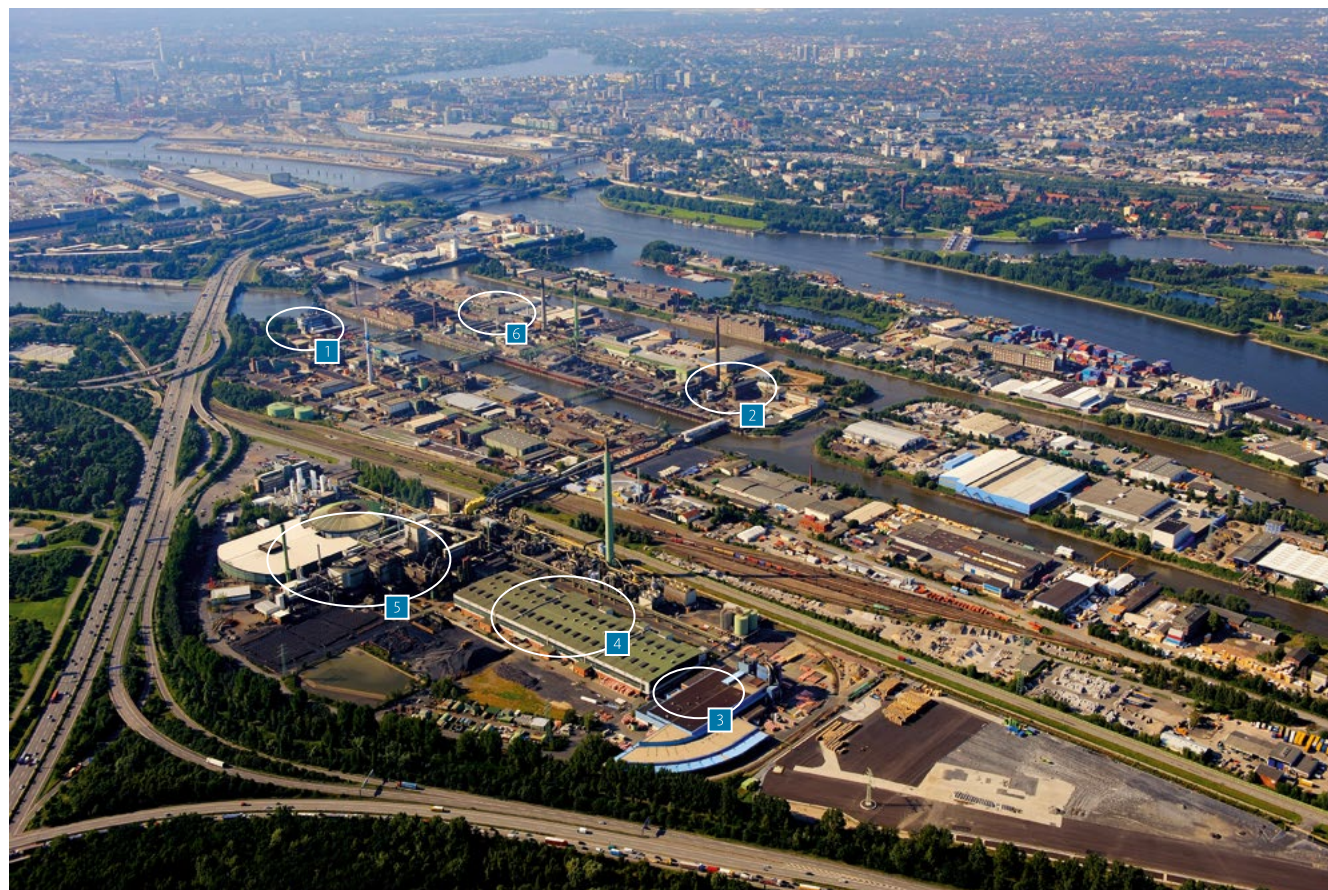
1 Continuous casting plant 2 Secondary copper smelter/precious metals 3 Rod plant 4 Tankhouse 5 Primary smelter (RWO) 6 Administrative building
